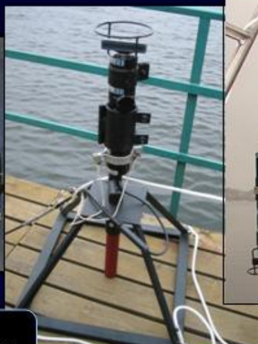
VDS – Variable Depth Sonar
